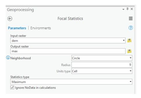
You will now need to find the minimum elevation value in a circular radius of 9 cells around each cell.
