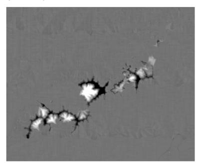
You will now generate a classification of the terrain change using the **Reclassify Tool**. In this model, we will assume that changes of less than 4 meters represent no change (e.g. background noise).
