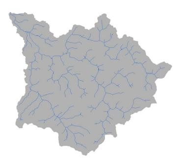
This calculation will produce a binary raster in which 1 represents pixels that were selected as streams and 0 represents non-stream pixels. You will now need to reclassify the 0 pixels to NoData using the Reclassify Tool.
