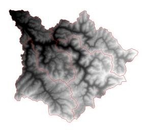
We will start our analysis by filling in the DEM. Note that this is not always necessary since some DEMs have already been filled or are hydrologically corrected. This operation can take some time to complete on a large DEM.
