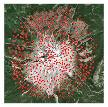
The points represent discrete elevation measurements. However, we would like a space filling surface that provides an elevation estimate at all locations. So, the points will be used to generate a TIN.
